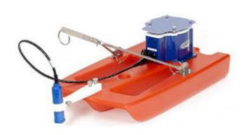
The GEO-StreamPro's transducer can be towed from different points onboard the platform, or can be removed and hand held in the water for applications such as under ice flow measurements.
